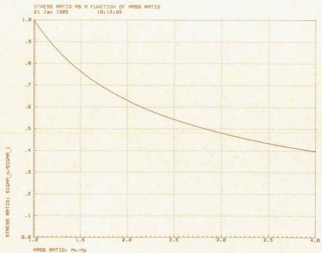
Fig. 3. Stress ratio versus ratio of counterweight mass to printbar mass. Stress ratio is the stress in the counterweight flexures for a given mass ratio divided by the stress for a mass ratio of one.
